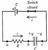
When the switch is closed, the charge on the capacitor increases over time while the current decreases.
